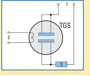
1 = Circuit voltage 2 = Heating voltage 3 = Load resistor
