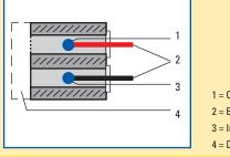
1 = Catalyzer pellistor 2 = Electric connections 3 = Inert pellistor 4 = Diffusion filter
