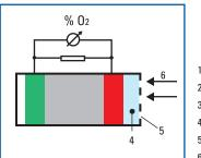
1 = Anode 2 = Electrolyte 3 = Cathode 4 = Diffusion path 5 = Diffusion filter
