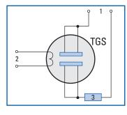
1 = Circuit voltage 2 = Heating voltage 3 = Load resistor
