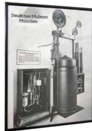
The first automatic flue gas monitor "ADOS" from 1900. Driven by updraught in the chimney, the unit takes a sample of flue gas 10-times per hour, automatically analyses the sample and records the content of carbon dioxide. This forms a measure for the most economic use of fuel by the personnel responsible (boilermen). The standard is around 15% carbon dioxide content in the furnace gases.
