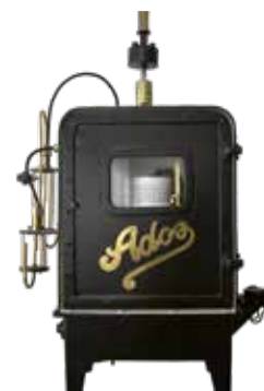
A test instrument hanging in an universal joint (to compensate the strong wave motion on board of a ship), when measuring carbon dioxide.
