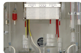
Triple test instrument (Triplex) for monitoring the CO, H 2 and CO 2 content of the ambient air. Used in the chemical industry.
