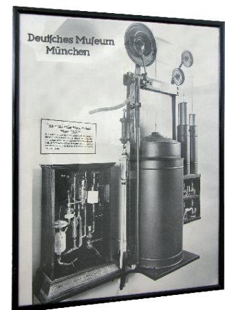
The first automatic flue gas monitor "ADOS" from 1900: Driven by updraught in the chimney, the unit takes a sample of flue gas 10-times per hour, automatically analyses the sample and records the content of carbon dioxide. This forms a measure for the most economic use of fuel by the personnel responsible (boilermen). The standard is around 15% carbon dioxide content in the furnace gases.
